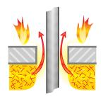
The temperatures inside a process heater can reach 2000°F and above. In instances of draft fan failures, this heat may cause extreme damage to a furnace penthouse. Nextel fiber can withstand direct flame impingement and prevent flame penetration.
