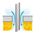
A draft fan  $\Delta P$  of 0.35" of water draws outside air through a nominal 1 ft<sup>2</sup> gap at a rate of 1.92 lbs/sec., every day, every month, every year. Tube seals made using Nextel ceramic textiles help stop the ingress of air.
