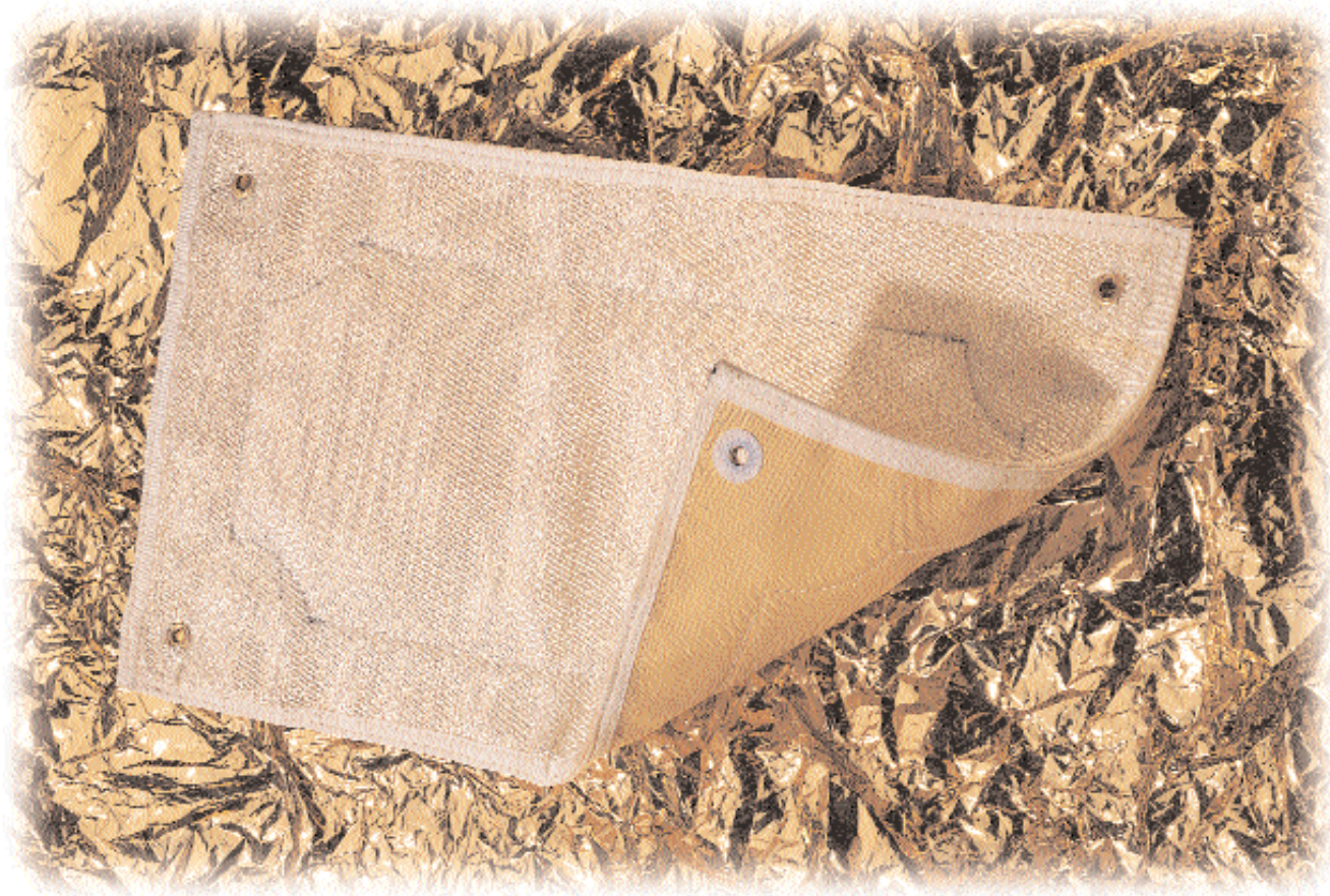
Top: The Stuffed Whipple Shield offers greater protection and requires less space in protecting spacecraft from being disabled by collisions with space debris, similar to what is shown at left. The shield, produced at NASA Marshall Space Center in Huntsville, AL, and the Johnson Space Center in Houston, TX, contains 3M™ Nextel™ Ceramic Fabric. Nextel was shown to be a key component in the development of this lightweight improvement to conventional shielding.*
