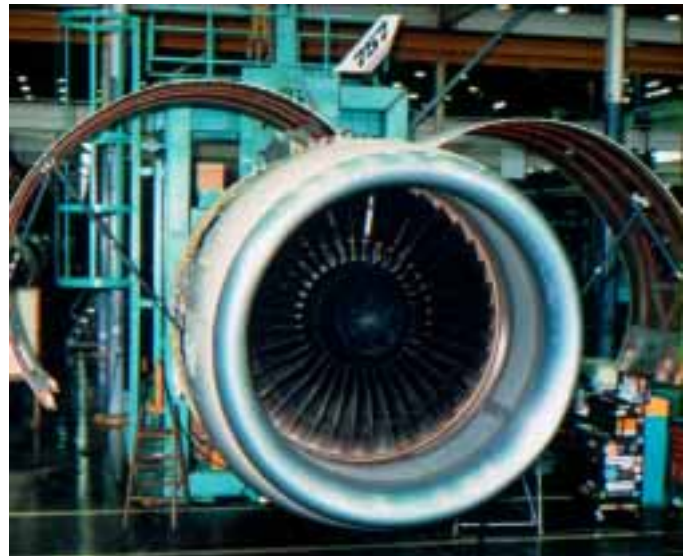
The Boeing 757's fan cowls are protected with a firewall blanket using a fabric of Nextel 312 Ceramic Fibers.
